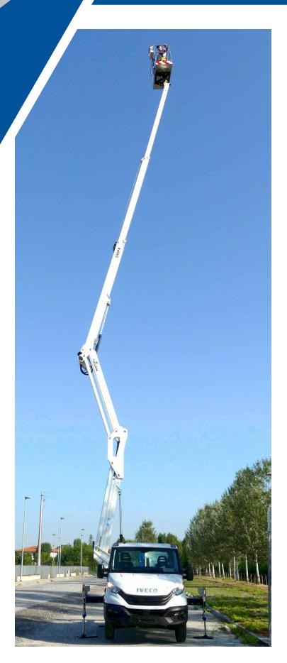
The GSR B240PX platform introduces a new feature in the concept of double "up-and-over" articulation.
