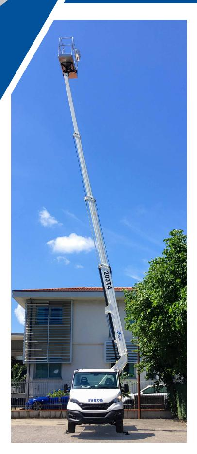
The GSR B200T4 platform reaches a new level in its telescopic range on 3,5t vehicles. While maintaining its traditional rigidity and sturdiness, this model introduces several significant elements of innovation offering improved outreach with reduced footprints.
