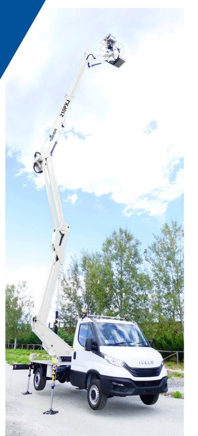
The new platform B210PXJ integrates the double up-and-over articulation with the final 2-meters JIB and the end-mounted basket. Sophisticated but simple, powerful and unrestricted, it allows to overcome obstacles at height with easy and intuitive manoeuvres.
