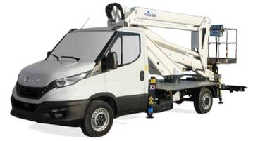
The GSR double articulated platform B240PX allows to reach a maximum horizontal outreach of 12,3 metres. This machine maintains the stabilization "in shape", with the result of being particularly compact.
