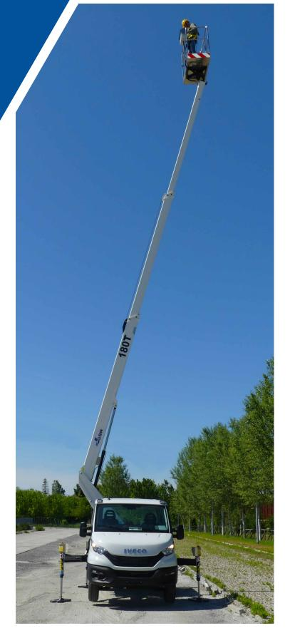
The new GSR B180T reaches a new level in its telescopic range on 3,5t vehicles.
