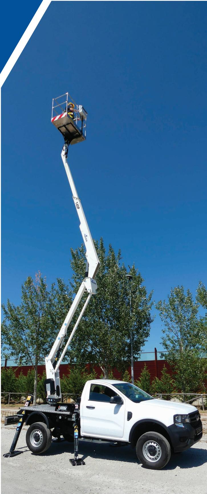
The E140P platform combines the traditional rigidity and robustness typical of GSR production with the versatility of the telescopic articulated boom. The final result is a compact and reliable machine. The particular geometry allows the installation on pick-up, allowing to reach work areas that are inaccessible to traditional machines.
