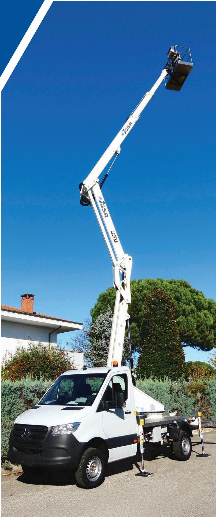
The GSR B220PXE platform integrates the double “up-and-over” articulation with an innovative telescopic boom and end mounted basket.
