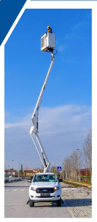
The GSR E140P platform combines the traditional rigidity and strenght with the versatility of the telescopic articulated boom. The result is a compact and reliable machine. The particular geometry allows the installation on pick-up, allowing to reach areas of work that are inaccessible to traditional machines.
