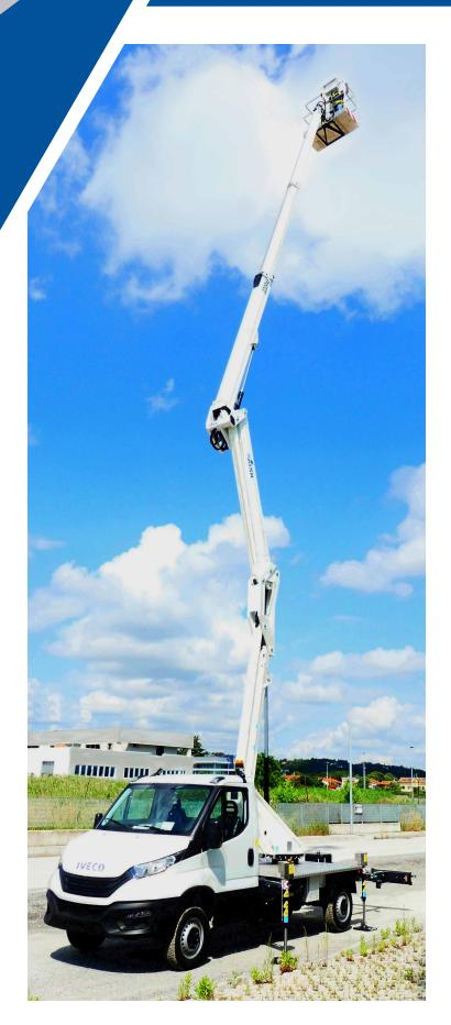
The new B220PXE platform integrates the double "up-and-over" articulation with an innovative telescopic boom and end mounted basket.
