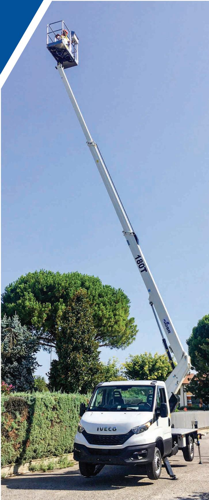
The GSR B180T platform reaches a new level in its telescopic range on 3,5 t vehicles.
