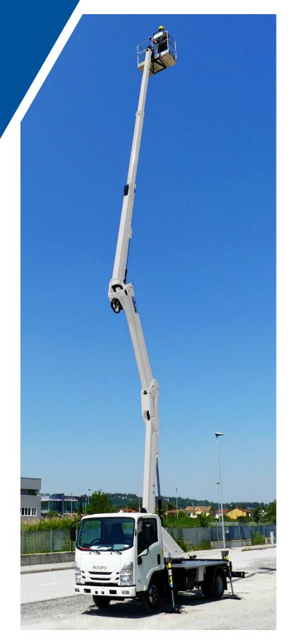
The GSR B220PXE platform integrates the double "up-and-over" articulation with an innovative telescopic boom and end mounted basket.
