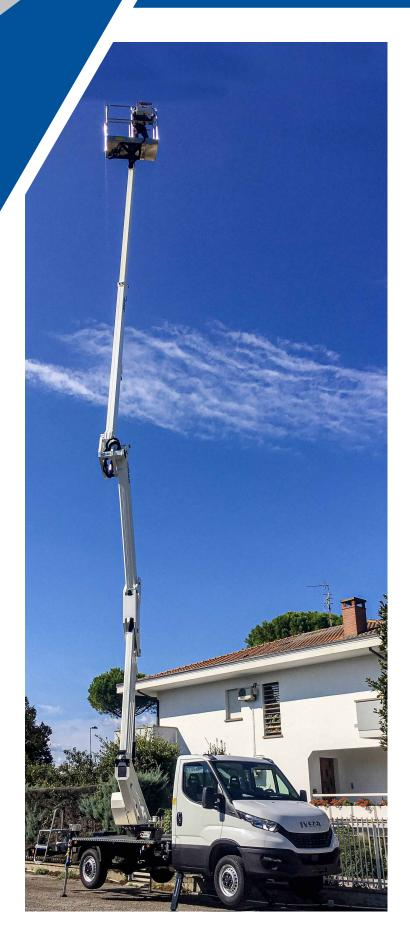
The GSR double articulated platform B200PX allows to reach a maximum horizontal outreach of 9 metres. This machine maintains the stabilization "in shape", with the result of being particularly compact.
