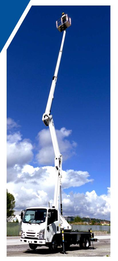
The GSR double articulated platform B240PX allows to reach a maximum horizontal outreach of 12,3 metres. This machine maintains the vertical stabilization "in shape", with the result of being particularly compact, also thanks to its length in running order of 6,52 metres only.
