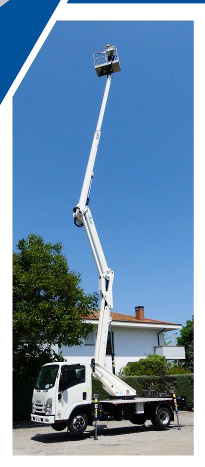
The GSR double articulated platform B200PX allows to reach a maximum horizontal outreach of 9,1 metres. This machine maintains the stabilization "in shape" with the result of being particularly compact, also thanks to its length in running order of 6,60 metres only.
